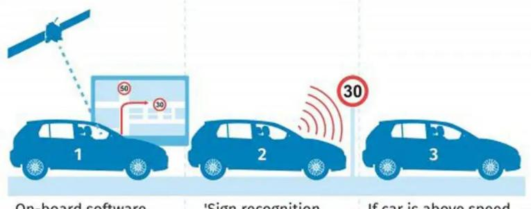
On-board software logs position of car using GPS data and digital map 'Sign recognition camera' also logs speed limit If car is above speed limit, warning sounds and vehicle slows down automatically
